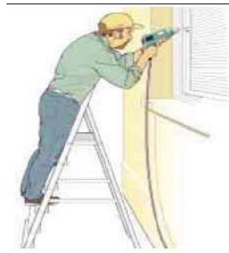
Correct – steps facing work activity
